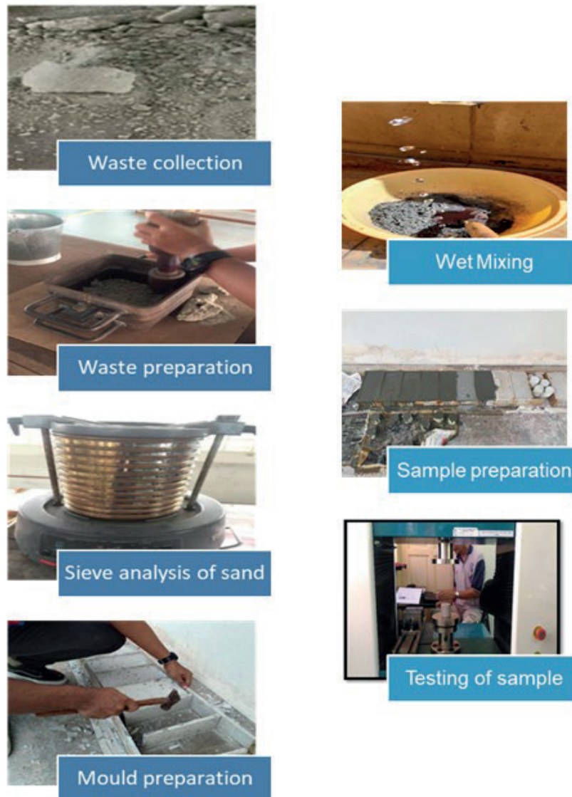
Fig. 1. Experimental Study on Recycling Foundry Waste into Bricks
