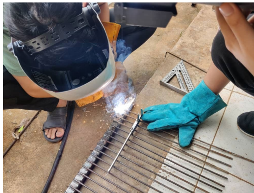
Figure 9: Weldment process of rake
